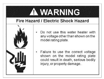
Before making the conversion to 5500 watts, check the (1) power supply . . . must be 240 volts, (2) wiring . . . 10 gauge AWG @ Type TW, 60°C or equivalent, and (3) Circuit breakers or fusing . . .capable of 30 amp loading. Also, the installation must conform with this manual, local codes and electric utility rules. Failure to comply can result in DEATH, SERIOUS BODILY INJURY, OR PROPERTY DAMAGE.
